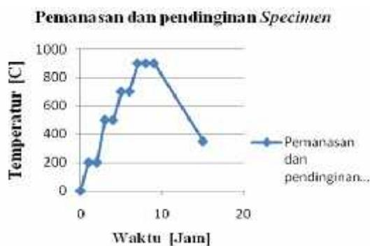
Gambar 1. Proses pack carburizing.
